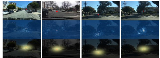
Fig. 6. Samples leading to erroneous decisions and their attributions. When red circle perturbations are introduced, the model mistakenly decides to initiate a braking action. The attribution maps confirm that these misjudgments are directly influenced by the perturbations, indicating a bias of the model to specific visual stimuli that can lead to incorrect responses.
